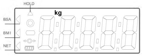
**BSA**: Body Surface Area is being displayed **BMI**: Body Mass Index is being displayed **NET**: Net weight appears after tare is activated
