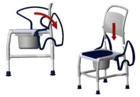
2. Swivel the armrests forwards until they click into the slots of the backrest and the locking pins click into the lower frame. Be sure they are securely in place.
