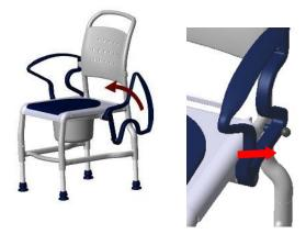
3. For chairs with height adjustment, the seat height of the chair is set at its lowest position for delivery (Base setting). Adjust the height as necessary (see: 10.7).
