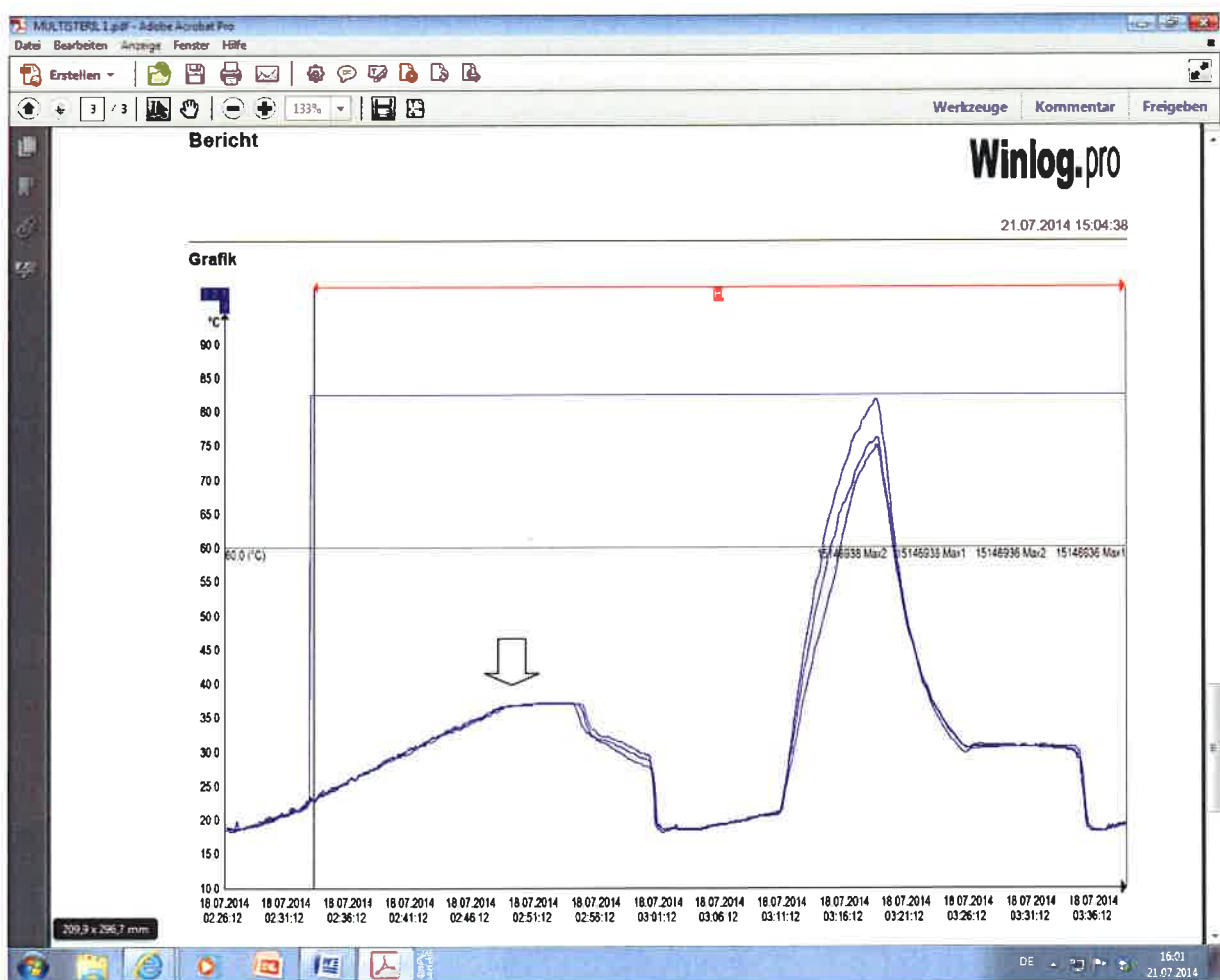
Figure 5: temperature profile of the liquid in the processing device (batch I)
